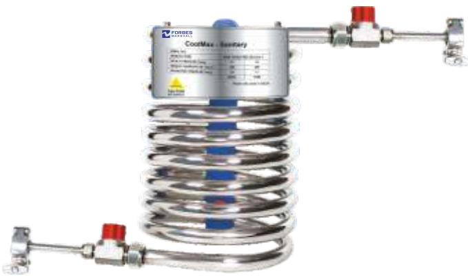
The Sample Cooler has a compact, space saving, shell-in-shell design which ensures quick and safe sampling of high purity media. A counter current flow is utilised to maximise cooler efficiency.
